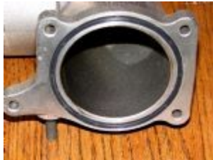
Stock elbow with O-Ring attached:
