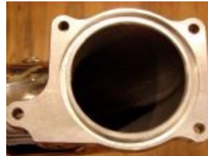
Power Air Inlet showing the groove for the reusable rubber O-Ring:
