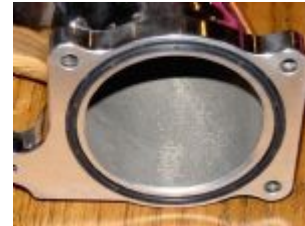
Power Air Inlet shown with rubber O-Ring installed:
